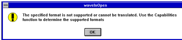
Figure 8. Message Box reporting an unavailable compression format or an invalid sample rate.
